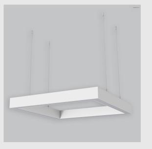
Viraj 45 Square has : •Square ring •Surface powder coat •Luminaire housing of aluminium •LED PCB mounted •Bottom opening for easy maintenance •Pendant with cable suspension •Quick mounting system •M6 bolt for M6 fastener •High performance double Prismatic diffuser •Uniform illumination •Energy-efficient LED with color rendering
